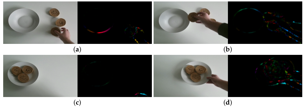
Figure 9. Visualization of Dense Optical Flow with Farneback: (a) moving ntakos, (b) moving ntakos inside the plate, (c) no move, (d) moving plate with ntakos.
